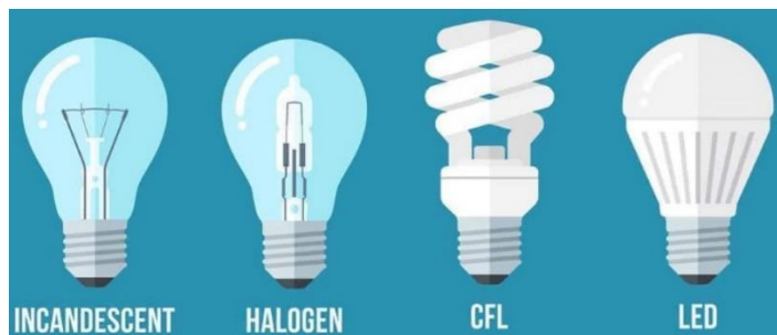
Fig. 1-4. Different types of light bulbs showing significantly increased energy efficiency from incandescent bulbs to halogen bulbs to compact fluorescent lamps (CFL) to light emitting diode (LED) bulbs
